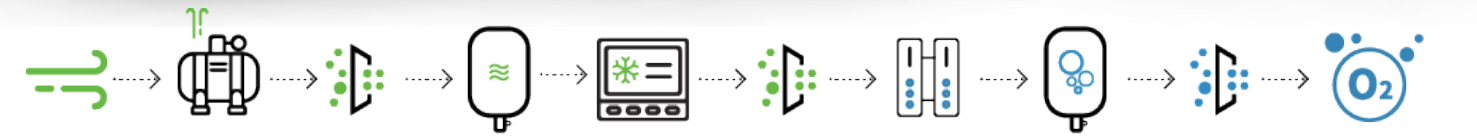
Schematic Diagram of Medical Molecular Sieve Oxygen Generator
